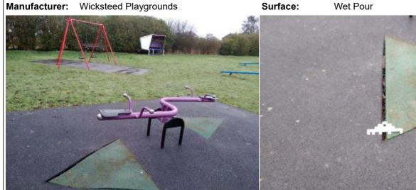
Finding: There are significant gaps (over 30mm) between the surface and the edging or between the joints in the surface; these are large enough for a small foot to enter
